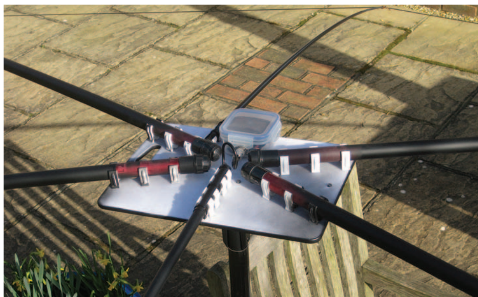
PHOTO 2: Close-up of the central spreader plate, which is key to the design.
