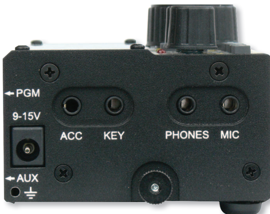
The KX2 end panel contains most sockets other than the BNC RF socket, which is on the other end.
