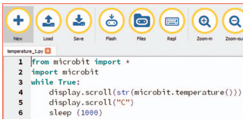
FIGURE 5: Code to scroll the micro:bit temperature across the screen every second.
